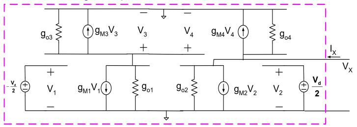
$$I_{\chi} = V_{\chi} (g_{02} + g_{04}) + g_{m2} \frac{V_{d}}{2} + g_{m4} V_{4}$$
