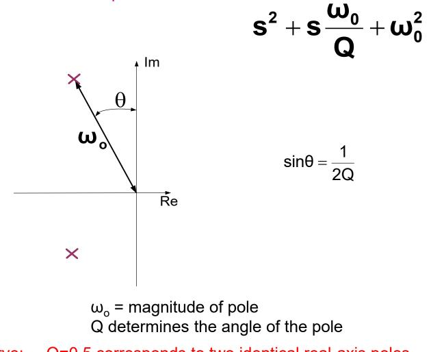
Observe: Q=0.5 corresponds to two identical real-axis poles Q=.707 corresponds to poles making 45° angle with Im axis
