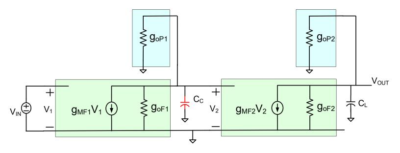
$$\begin{array}{l} V_{2}\left(sC_{C}+g_{_{OF1}}+g_{_{OP1}}\right)+g_{_{mF1}}V_{_{IN}}=0 \\ V_{_{OUT}}\left(sC_{_{L}}+g_{_{OP2}}+g_{_{OF2}}\right)+g_{_{mF2}}V_{_{2}}=0 \end{array} \right) \label{eq:V2}$$
