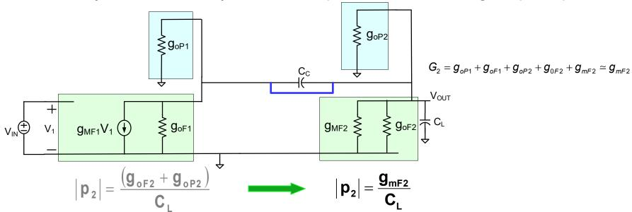
Will be shown later that C<sub>C</sub> introduces a zero in the gain function
