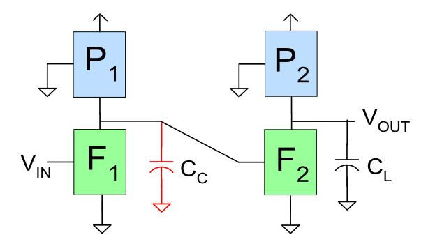
Consider single-ended input-output (differential analysis only slightly different) Can't get everything but can get most of the small-signal results Since internal node compensated, must have  $p_1 << p_2$
