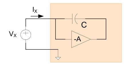
$$I_{X} = [V_{X} - (-AV_{X})] sC = V_{X} s [C(1+A)]$$
