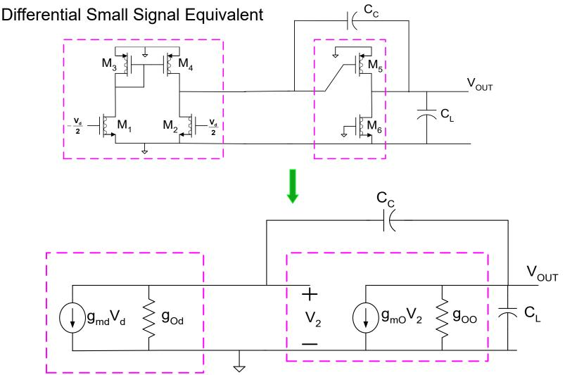
(This happens to be the general form for a two-stage structure with a quarter circuit and counterpart circuit !)
