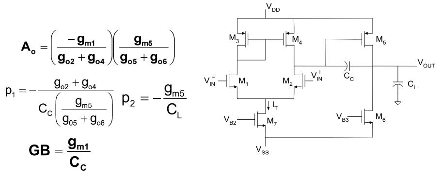
Note the simple results obtained from inspection agree with the more time consuming results obtained from a small signal analysis
