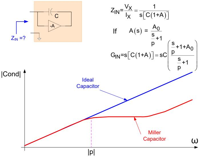
Does not behave as a capacitor for  $\omega > p$
