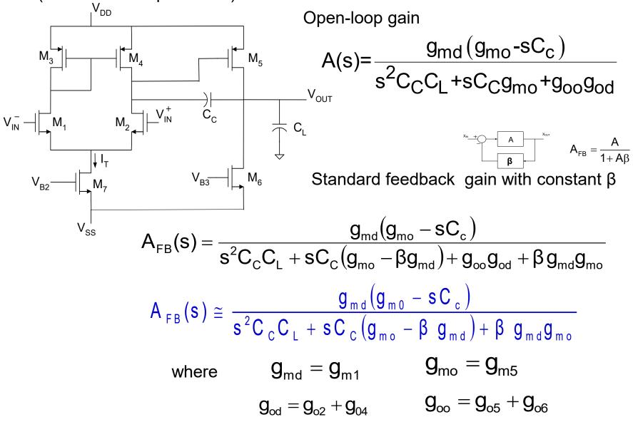
How does the Gain of the Two-Stage Miller-Compensated Op Amp Compare with Internal Compensated Op Amp with feedback  $A_{FB} = \frac{A}{1 + AB}$ ?
