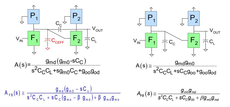
Internal node capacitor  $C_C$  or Miller  $C_C$  added externally Or "load compensation" before output buffer added externally
