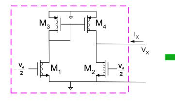
$I_{\chi} \cong V_{\chi} (g_{02} + g_{04}) + g_{m2} V_{d}$
