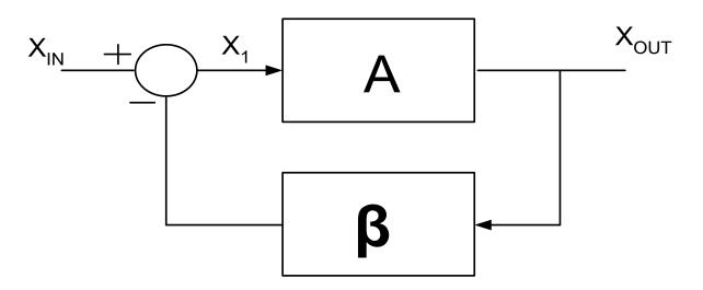
How does the amplifier perform with feedback?
